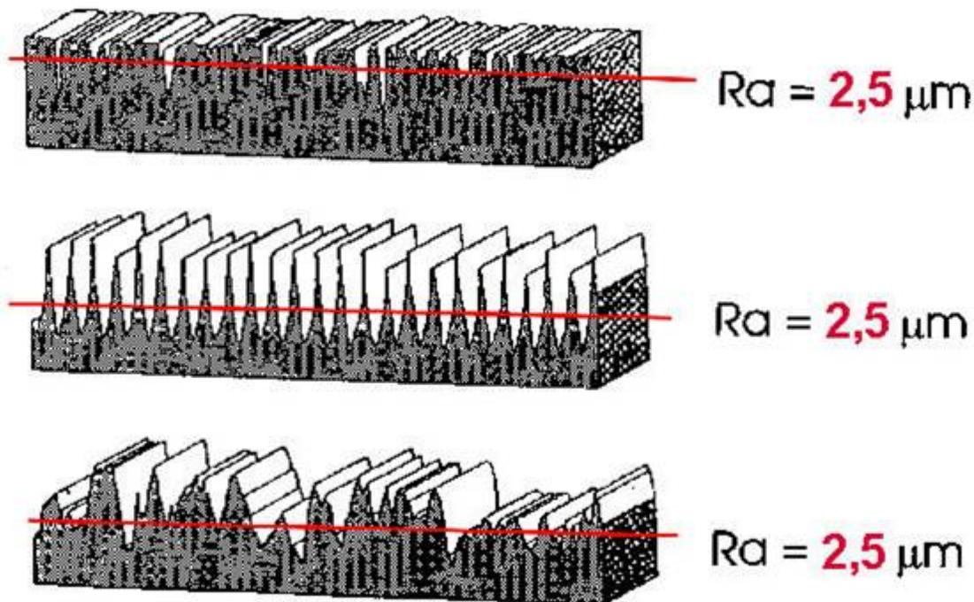
To fully characterize the shaft surface, two additional parameters should be observed.
